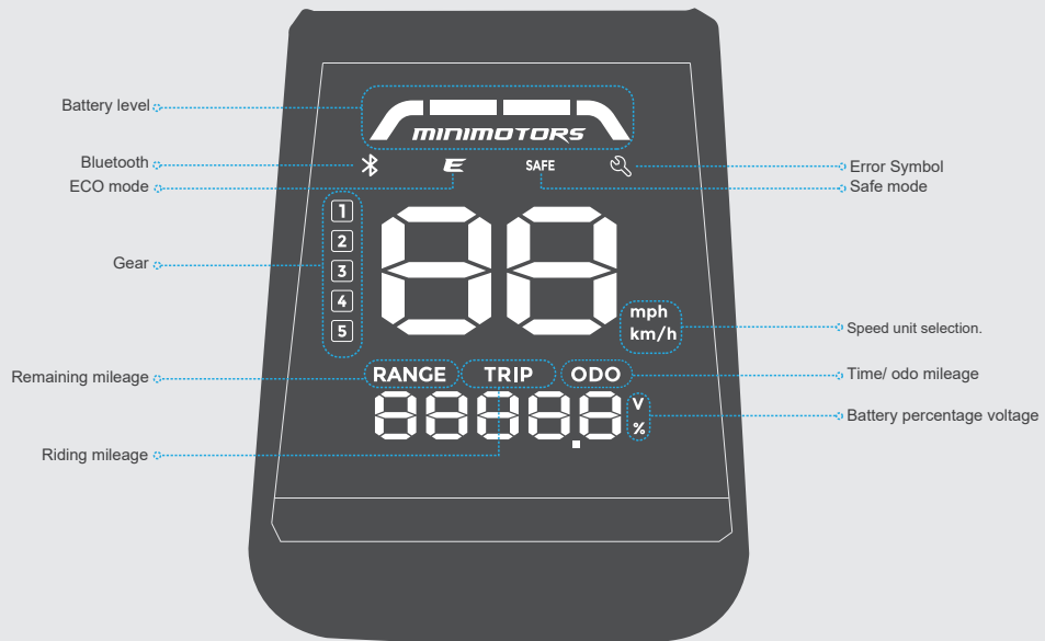
Minimotors EY2 smart digital screen (size: 47*50mm)
